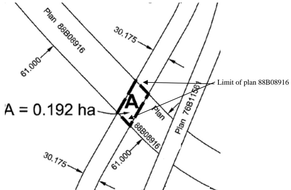
Plan 102189461 – A railway right of way was subdivided, creating Parcel A for a highway by using the limits of plan 88B08916.
